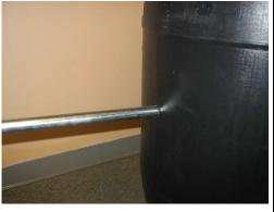
STEP 5: Install aluminum tube (short) into one side of barrel as shown. Slide aluminum tube up to PVC tube assembly. Lift and rotate PVC tube assembly and slide same aluminum tube through next hole down. Continue sliding aluminum tube through opposite side of barrel.
