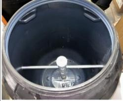
**STEP 6**: Rotate PVC tube so aluminum tube is 90 degrees to the through hole in barrel as shown.
